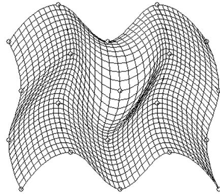
**Fig. 4 – A weights of 0.5 is assigned to the internal point of the surface**
