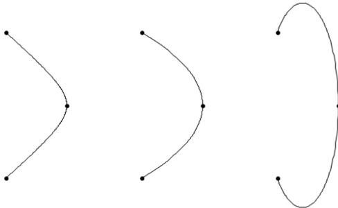
**Fig. 2 – Shape of spline curves depending on weights**
